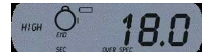
Time the internal sensor spent over specifications. High alarm is on, battery is low, Trip has ended.
