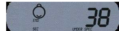
Time the internal sensor spent under lower alarm specification at the end of the logging cycle
