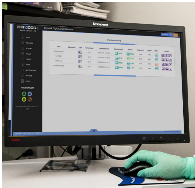
Cryopak's Mirador™ software provides device summaries through its intuitive interface
