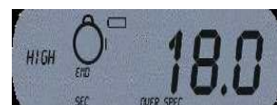
Time the internal sensor spent over specifications. High alarm is on, battery is low, Trip has ended.
