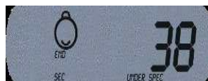
Time the internal sensor spent under lower alarm specification at the end of the logging cycle
