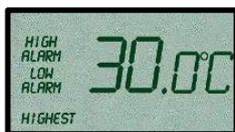
LCD displays the highest recorded reading
