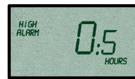
LCD displays the time above the specified high alarm setting for the current trip
