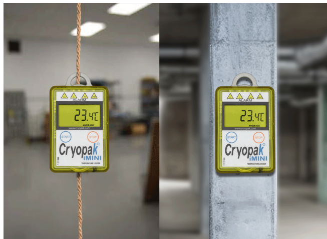
Figure 1: Installation of data loggers, hanging from rope in open spaces and attached to stationary objects.
